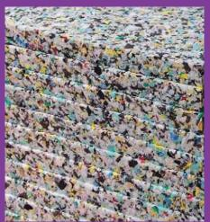
**SBR (Styrene Butadiene) Rubber:** It is a synthetic rubber derived from styrene and butadiene. It is suitable for use within the temperature range between -50 °C and +100 °C.
