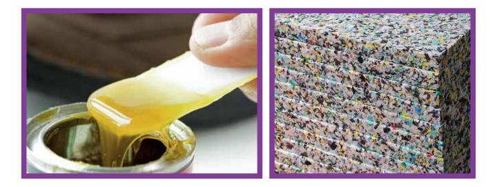
**SBR (Styrene Butadiene) Rubber:** It is a synthetic rubber derived from styrene and butadiene. It is suitable for use within the temperature range between -50 °C and +100 °C.
